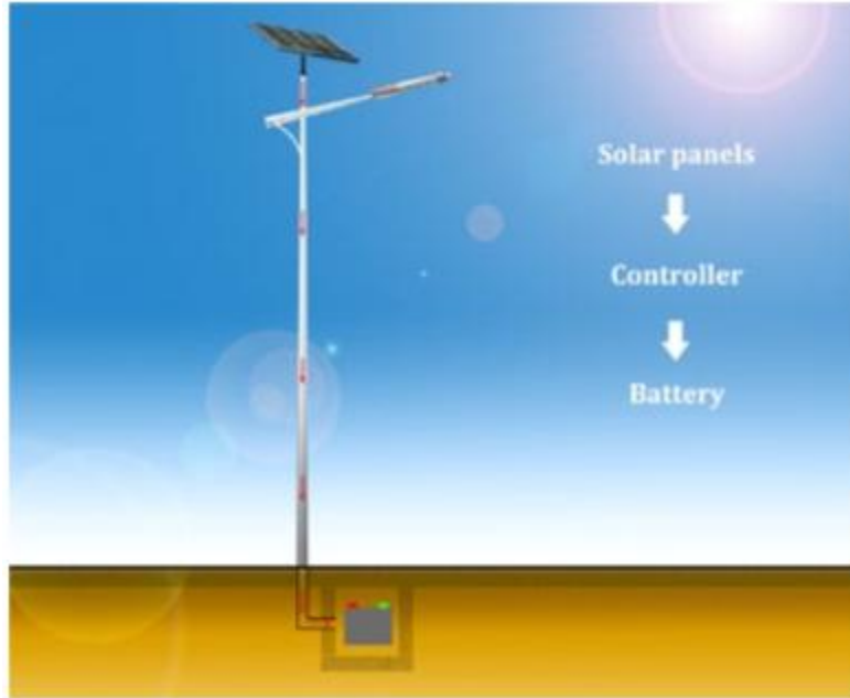
Solar panel charge the battery during the day
