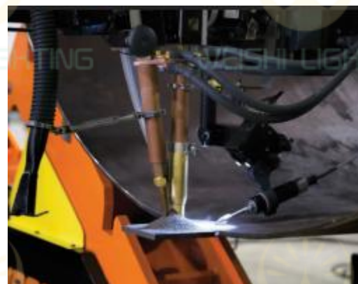
Automatic Full Welding and One-time Shaping
